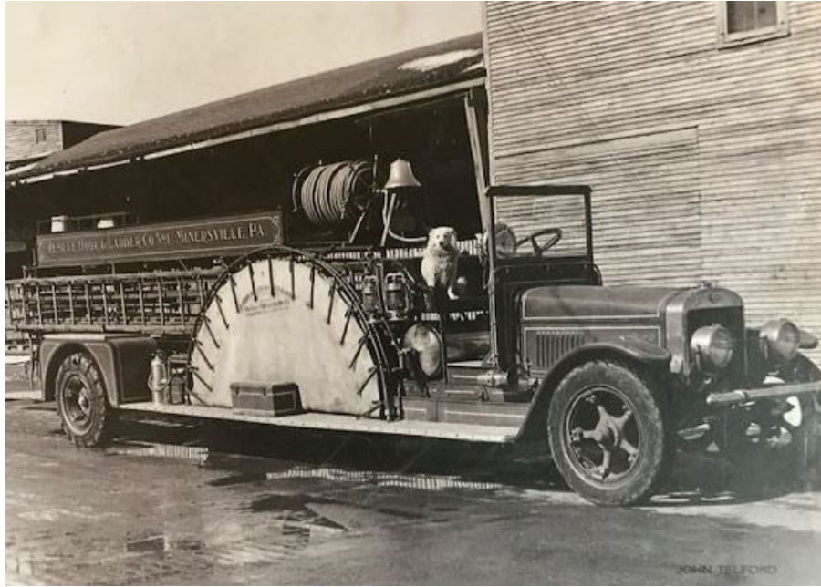
Rescue H & L of Minersville combination city service hook and ladder truck that was originally a 1915 American LaFrance Type 14 with a 40 gallon chemical tank and 235' of ground ladders.
