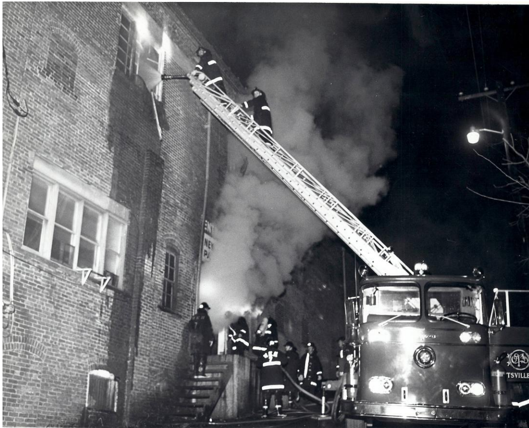
West End's 1960 Seagrave 65'/750 gpm quint has the ladder pipe in service at the Evans Moving & Storage/New Penn Paper fire in 1973.
